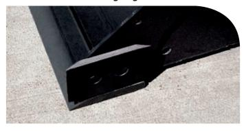
Add life to the high-wear corners of your bucket by bolting on corner cutting edges. Most Bobcat buckets have pre-drilled holes to accept bolt-on corner cutting edges.
