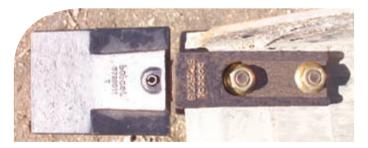
The 102 mm wide Hensley bucket tooth provides additional wear surface and reduces the rate of wear at the bucket edge and corners.
