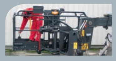
Just 10 seconds to slide the platform extensions into position and lock them through spring pins for safe use!
