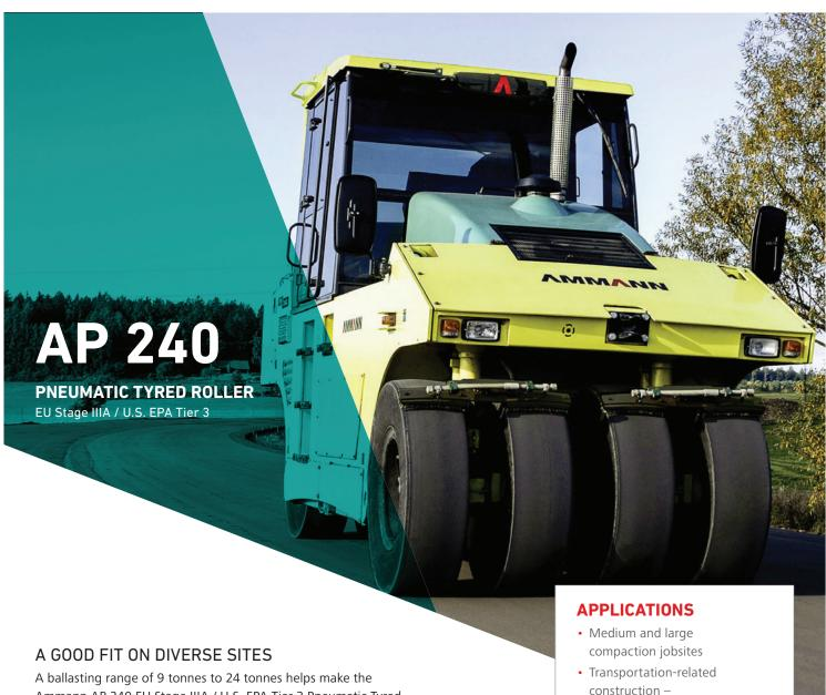
Ammann AP 240 EU Stage IIIA / U.S. EPA Tier 3 Pneumatic Tyred Roller a good fit on diverse jobsites. Also helping with flexibility is the Air-on-run system, which the operator uses to adjust tyre pressure without ever leaving the cab. Ammann Traction Control (ATC) boosts productivity on tough terrain. The proven hydrodynamic propulsion system provides power, while quality Ammann components and engineering enable reliability and long life.
